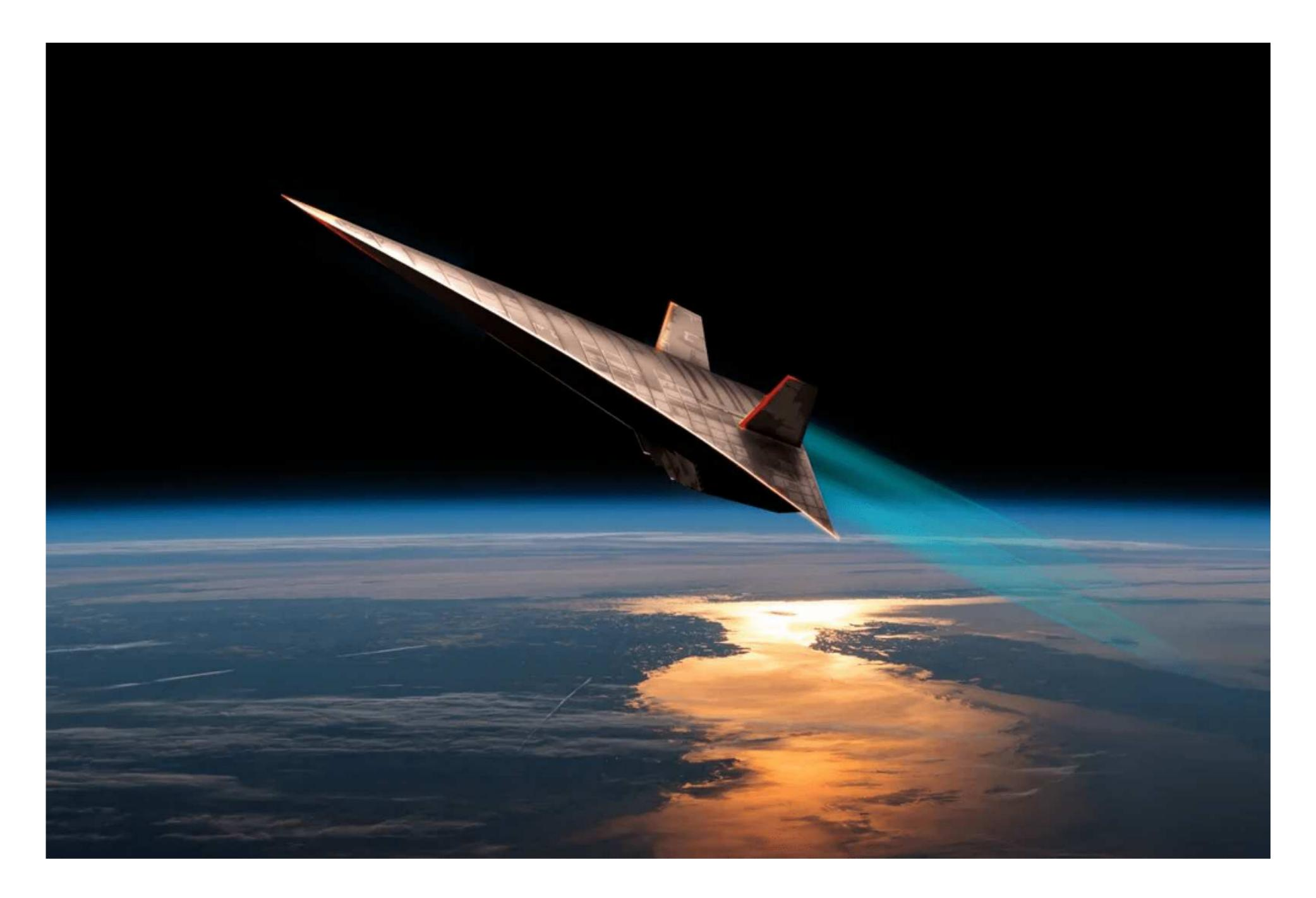
Ramjets and scramjets are types of air-breathing engines designed for high-speed flight, particularly at hypersonic speeds (Mach 5 and above). These engines operate on the principle of compressing incoming air without the need for traditional rotating compressors, as seen in turbofan and
