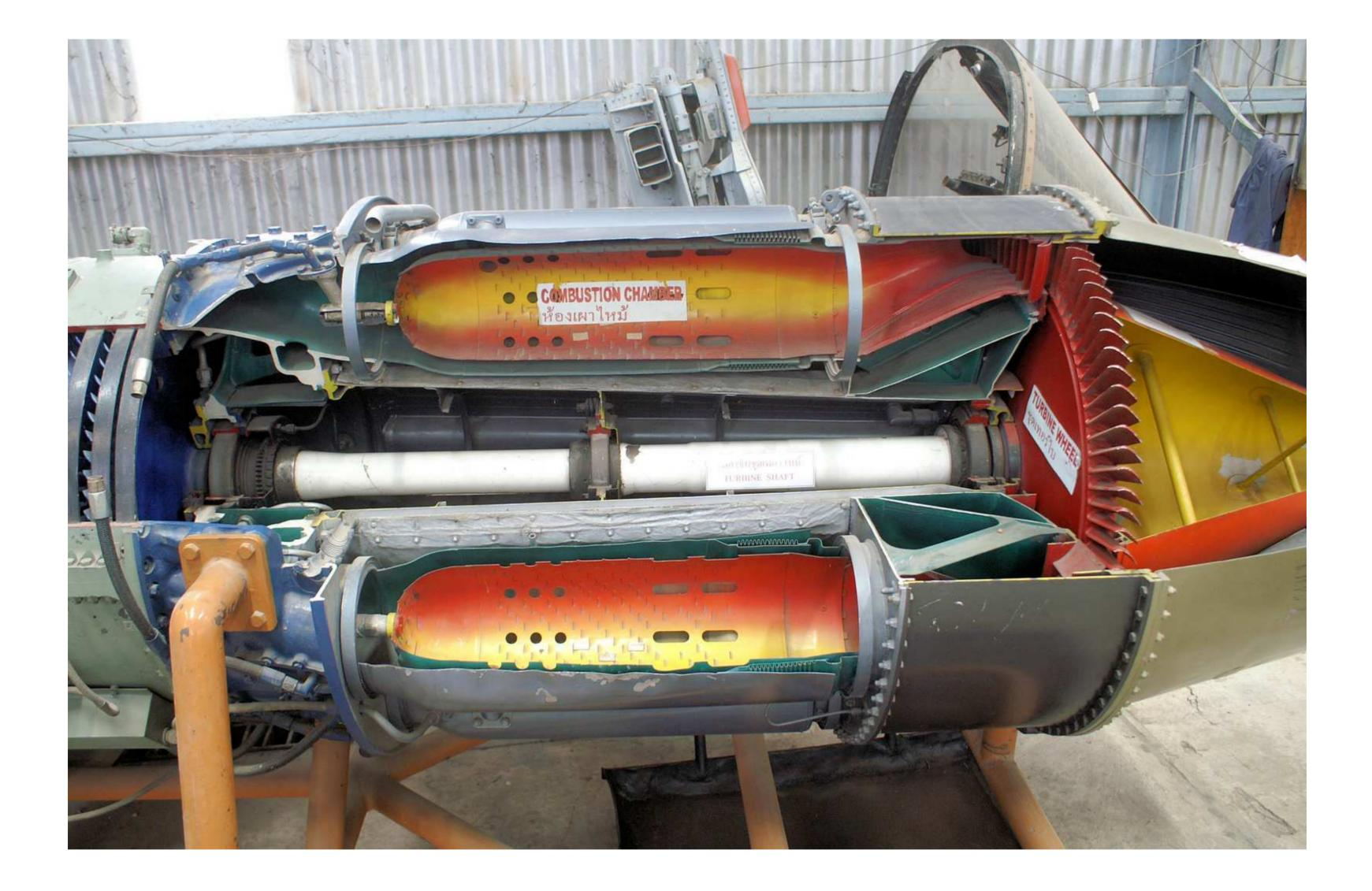
Operation: Fuel is injected into the combustion chamber, and it is ignited, often by spark plugs or igniters. The resulting combustion process raises the temperature and pressure of the air, creating a high-speed stream of hot gases.
