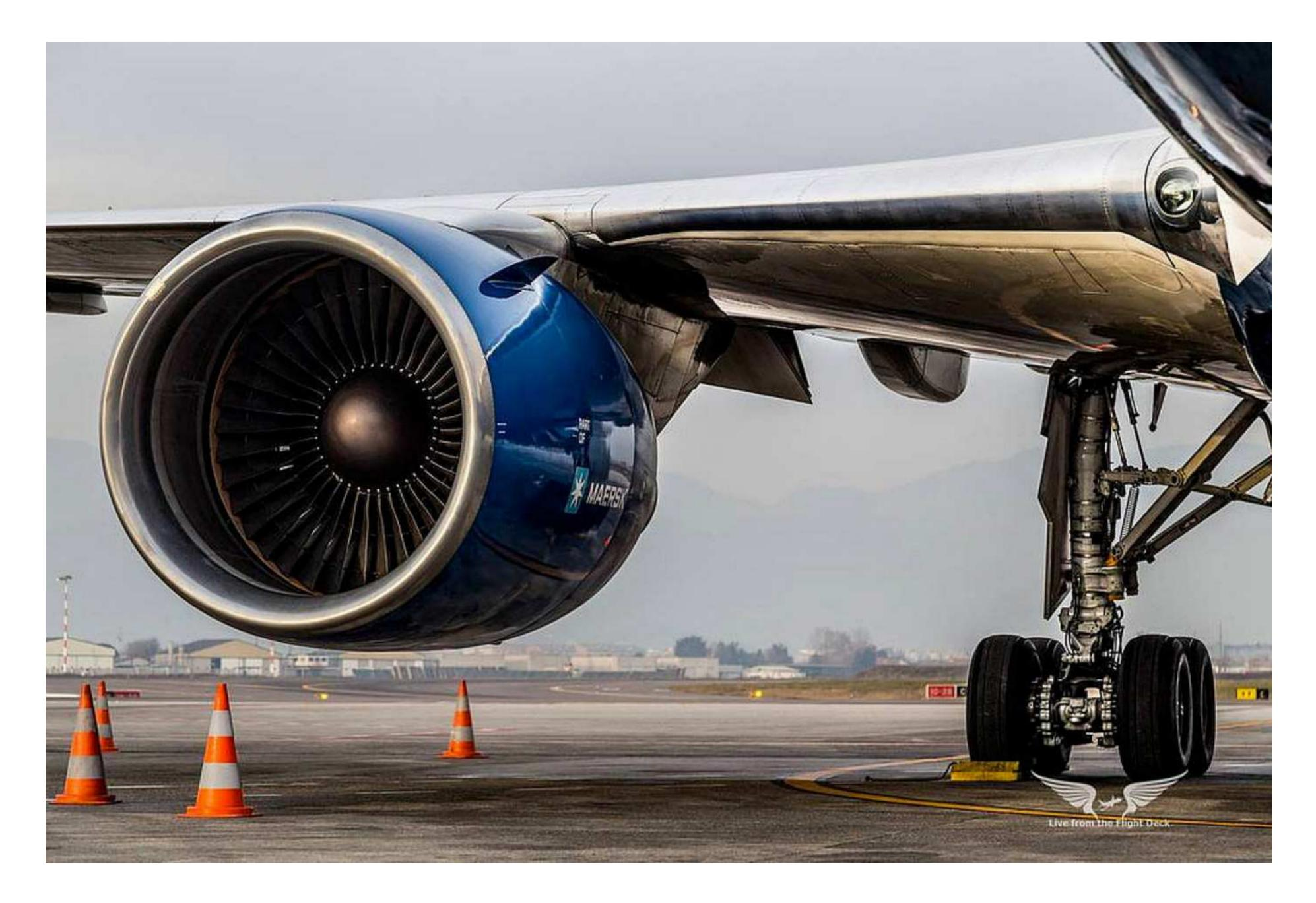
Turbofan engines, often referred to as "jet engines," are the most common type of propulsion system used in modern commercial and military aircraft. They offer a balance between speed, efficiency, and power, making them suitable for a wide range of aviation applications. Here's an overview of turbofan engines: Nozzle: The high-speed exhaust gases are expelled through a nozzle at the rear of the engine, creating forward thrust according to Newton's third law of motion.
