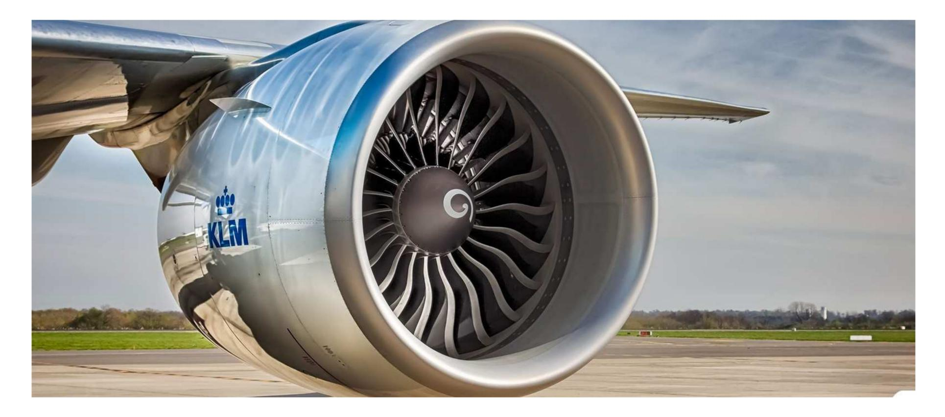
Operation: Air enters the engine through the inlet, and it is typically designed to slow down and compress the incoming air slightly to enhance engine efficiency.
