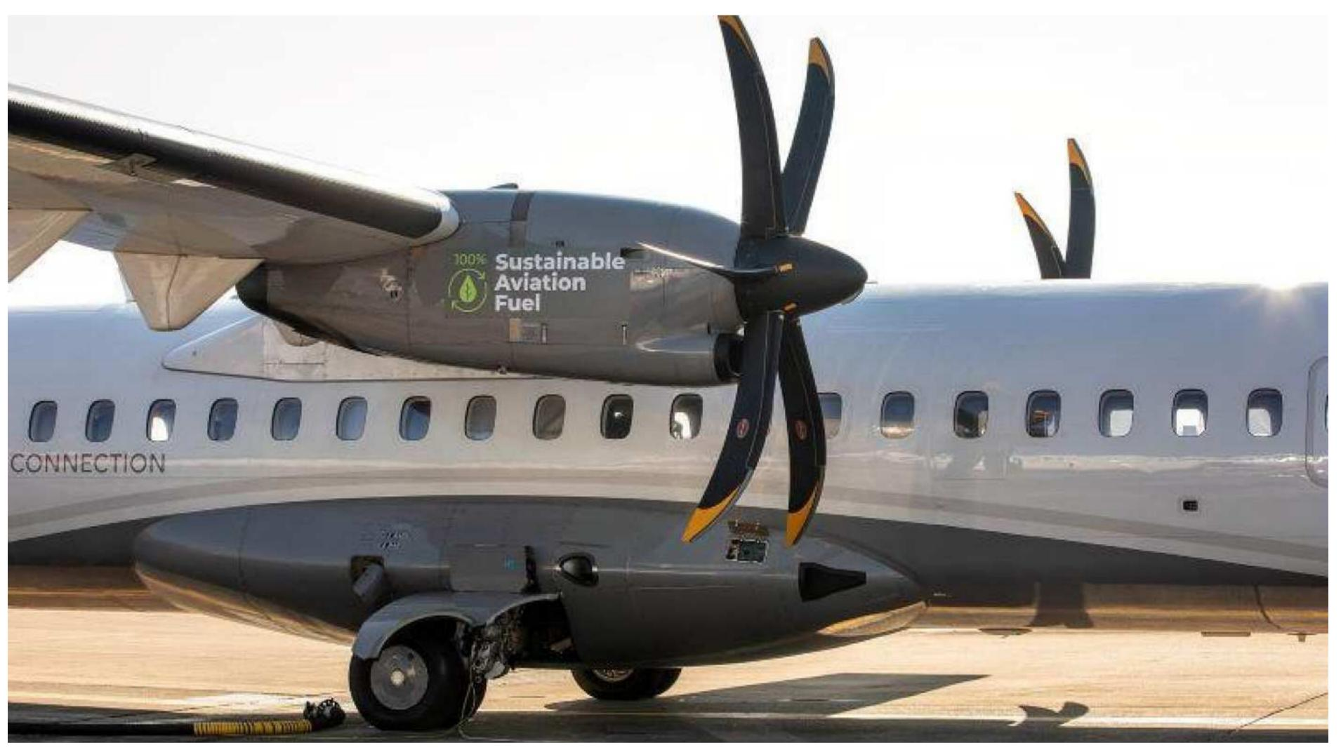
Turboprop engines, often simply referred to as "turboprops," are a type of aircraft propulsion system that combines elements of both jet engines and traditional piston engines. These engines are commonly used in regional and smaller aircraft where a balance between speed, efficiency, and short takeoff and landing (STOL) capability is important. Here's an overview of turboprop engines in aviation:
